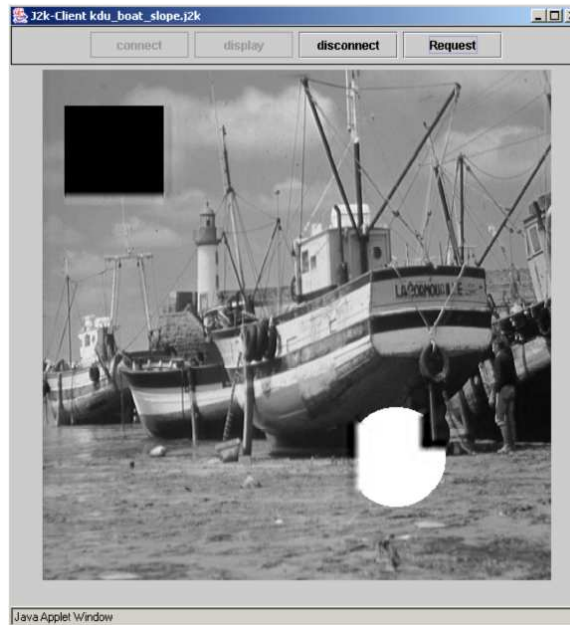
Figure E.11: The application of a high threshold value (Shown example: 10%) can impose artifacts or even lead to the neglect of elements containing modified contents (src: [Sch03a]).
