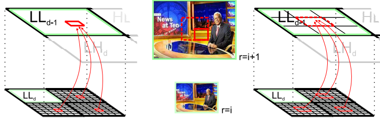
Figure 2.7: Reconstruction of a local area in decomposition level ( d-1 ) by using single code-block (left), or precinct structures (right) from level d . It can be seen that a precinct (dashed line) may contain more than one code-block.
